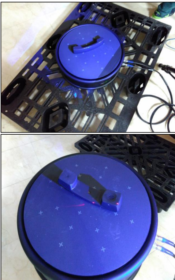
Fig 2: Scanning the Receiver From Different Views for the Registration by Using Structured Light
