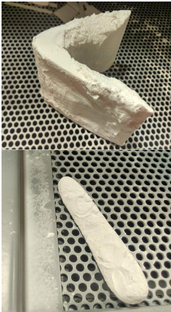
Fig 9: Prototype of the Base and Receiver Before Cleaning and Post-Processing
